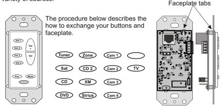
1 Detach the existing faceplate by pressing the plastic tabs with a flat blade screwdriver. (Press inward and upward (1) at a 30 degree angle)
